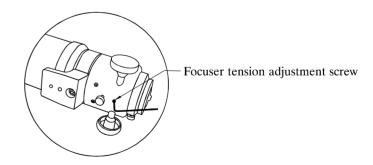
Focuser tension can be adjust using allen screw only when necessary. Please consult with William Optics dealer or manufacture for any uncertainty before making adjustment.
