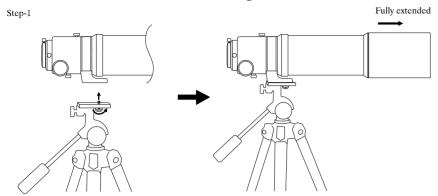
Connecting point between MEGREZ 80 ( L-bracket ) and commercial tripod . Carefully lock down the knob beneath before operation.
